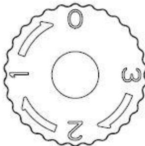
To control the internal temperature, adjust the control knob according to the ambient temperature or purpose of use.
